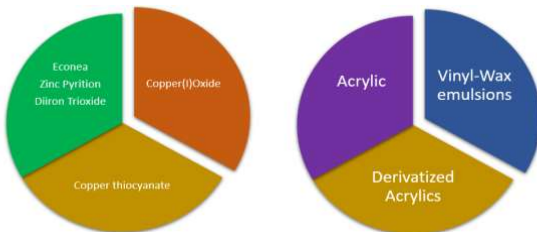
Figure 4. Main ingredients in commercial antifouling coatings for aquaculture applications
