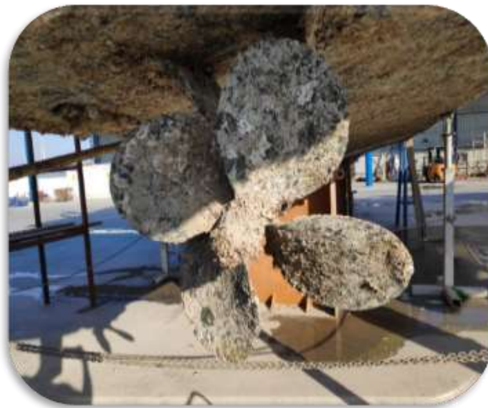
Figure 2. A ship's propeller coated with calcified products associated with marine biofouling.
